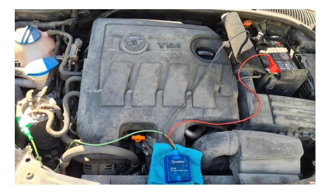
The green light will flash rapidly. After the set delay time has elapsed the measurement starts, the red light will flash once per set recording period.
