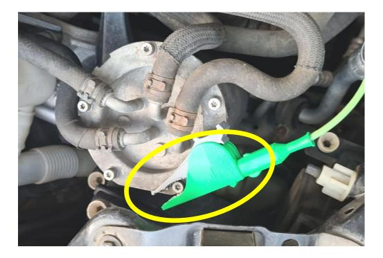
Attach the green crocodile clip to a suitable point on the car body or to another point conductively connected to the car body.
