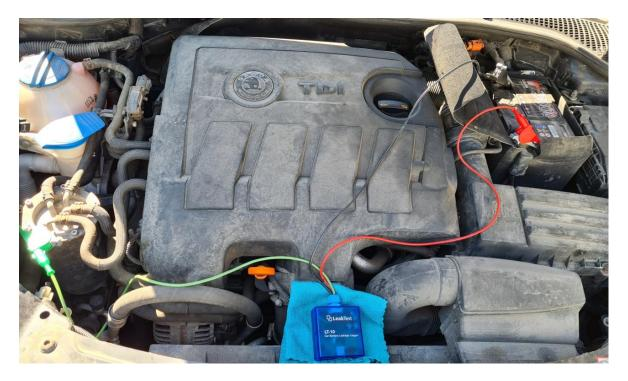
Disconnecting from the vehicle: unlock the vehicle and open the bonnet. The light on the Leaktest recorder no longer flashes. Disconnect the LeakTest - first the red, then the black and then the green crocodile clip.
